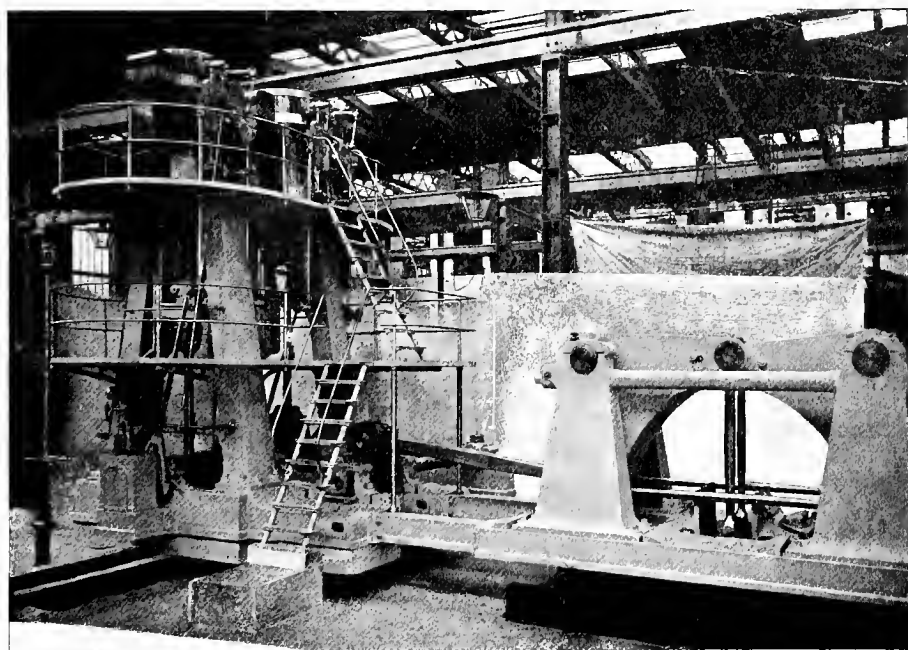
FIG. 82. VERTICAL COMPOUND PUMPING ENGINES WORKING TWO "ASHLEY" DEEP WELL PUMPS.
